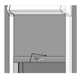
To lock the blind into position, rock the handle backwards.
