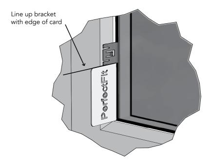
Line up the bracket with the base or top of the credit card (depending on which corner of the window you are working) and fit the bracket by pushing it between the glass and the rubber seal of the window.
