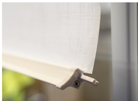
11. On opposite side, tilt bottombar to open position and slide side extrusion over bottombar end cap and fabric ensuring both are within the fabric channel on the side extrusion.
