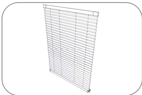
18. Hang blind for visual inspection and to check drop, where applicable set blind tension.
